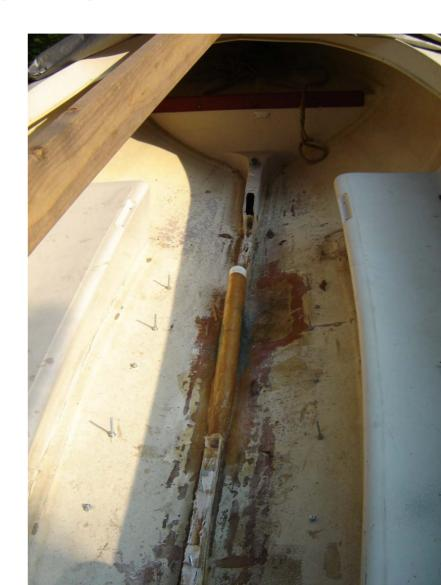
WITHOUT A KEEL, STEERING WOULD BE "SQUIRLEY", TWO ALUMINUM ANGLES (2 X 2 X 1/8) ARE BOLTED TO THE HULL, EACH ABOUT 1 FT FROM THE CENTERLINE OF THE BOAT. IN BIG SHIPS THESE ARE CALLED "BILGE KEELS". THE BOLTS THRU THE HULL WILL ALSO SECURE THE NEW DECK ON THE INSIDE OF THE HULL, THE MOTOR MOUNTS, AND THE STERN BEARING STRUTS FOR THE PROPELLER SHAFT
