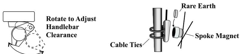
On the speedometer model, there is also a speed pickup cable and spoke magnet to detect the wheel rotation. The pickup attaches to the fork with two cable ties, and must be mounted to pass within 1mm of the magnet for the speed readings to function. The optional rare earth magnet is included that can be attached to the weaker ferrite magnet to allow for much greater clearance.
