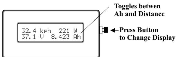
A quick press of the button will toggle to show other display screens of interest. The 2nd display shows just the electrical statistics from the battery pack, including the current in amps. This is the default screen for the non-speedometer model.
