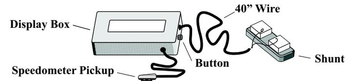
For operation, the shunt must be connected directly in series with the negative leads of your vehicle's battery pack. The orange wire must connect to the positive battery connection. It is recommended that this positive connection is placed after any series switch or fuse so that the meter powers down when the pack is shut off.
