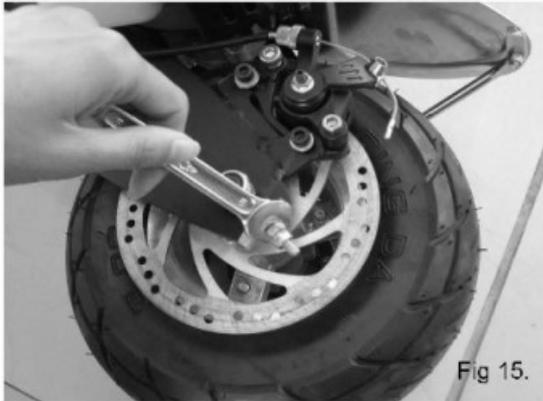
Occasionally rotate the rear wheel to make sure belt is aligned. Finally lock and tighten the rear axle bolts prior to riding.
