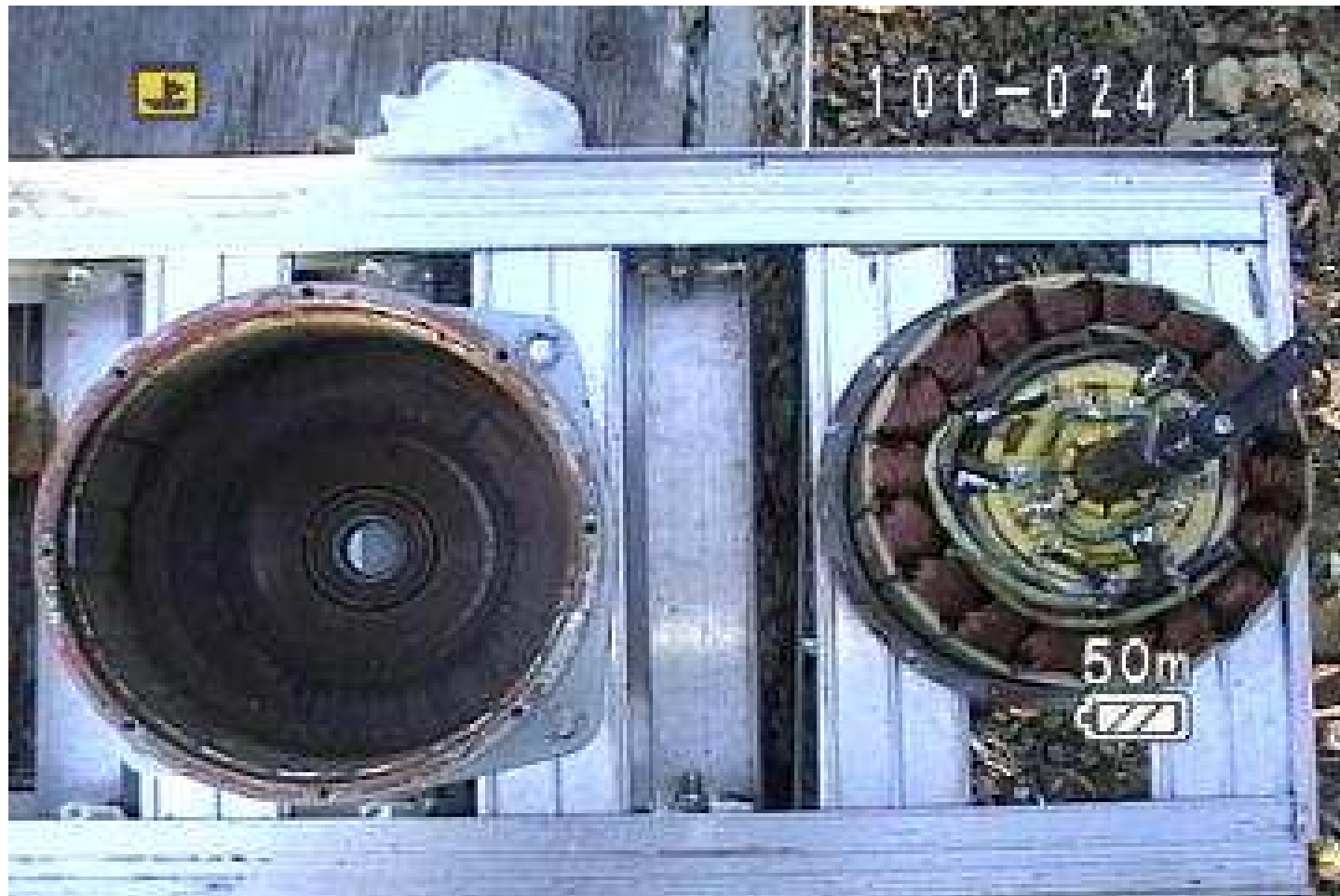
15 – The permanent magnet housing separated from the armature and cover plate.
