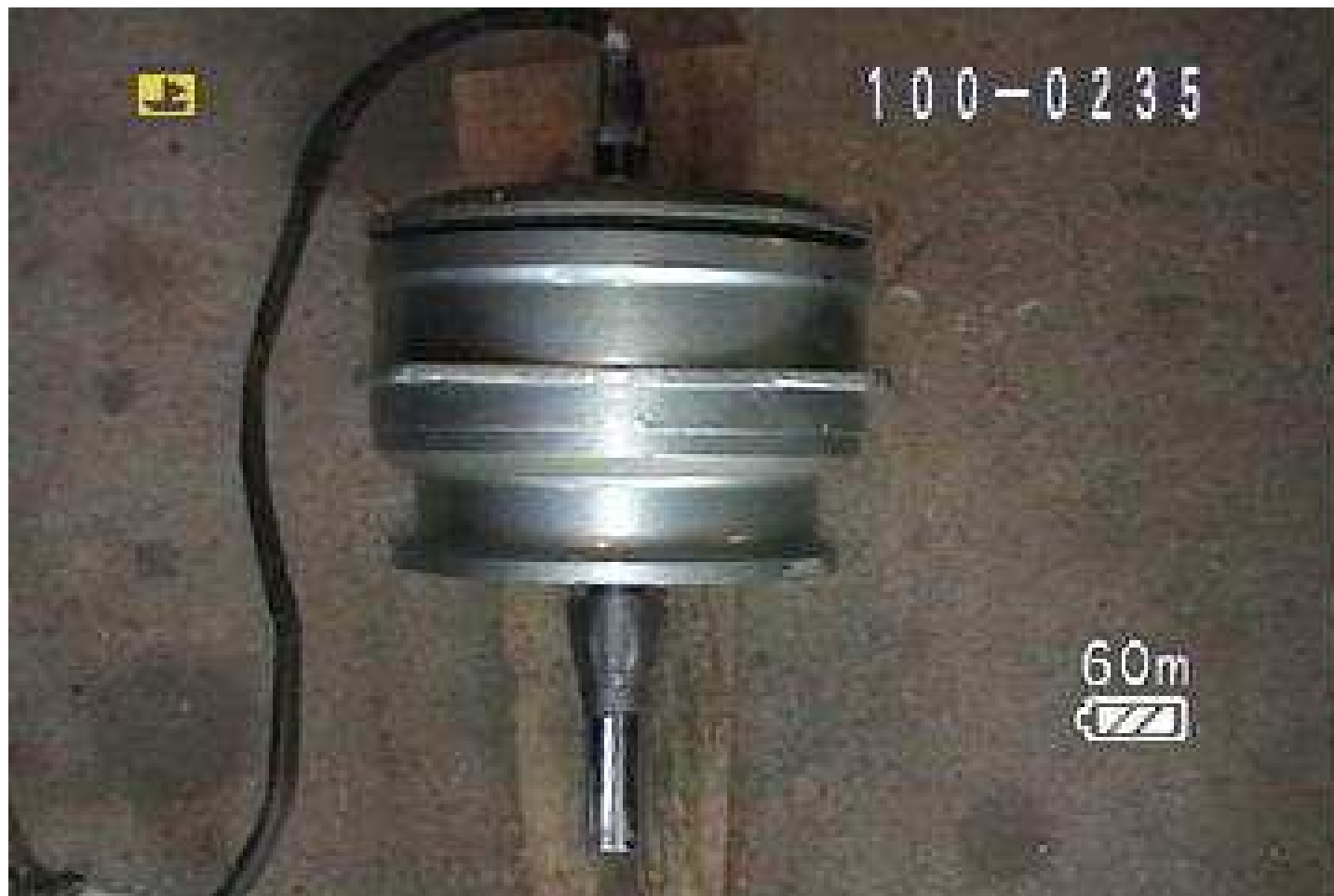
9 – Here you can see the housing is beginning to separate.
