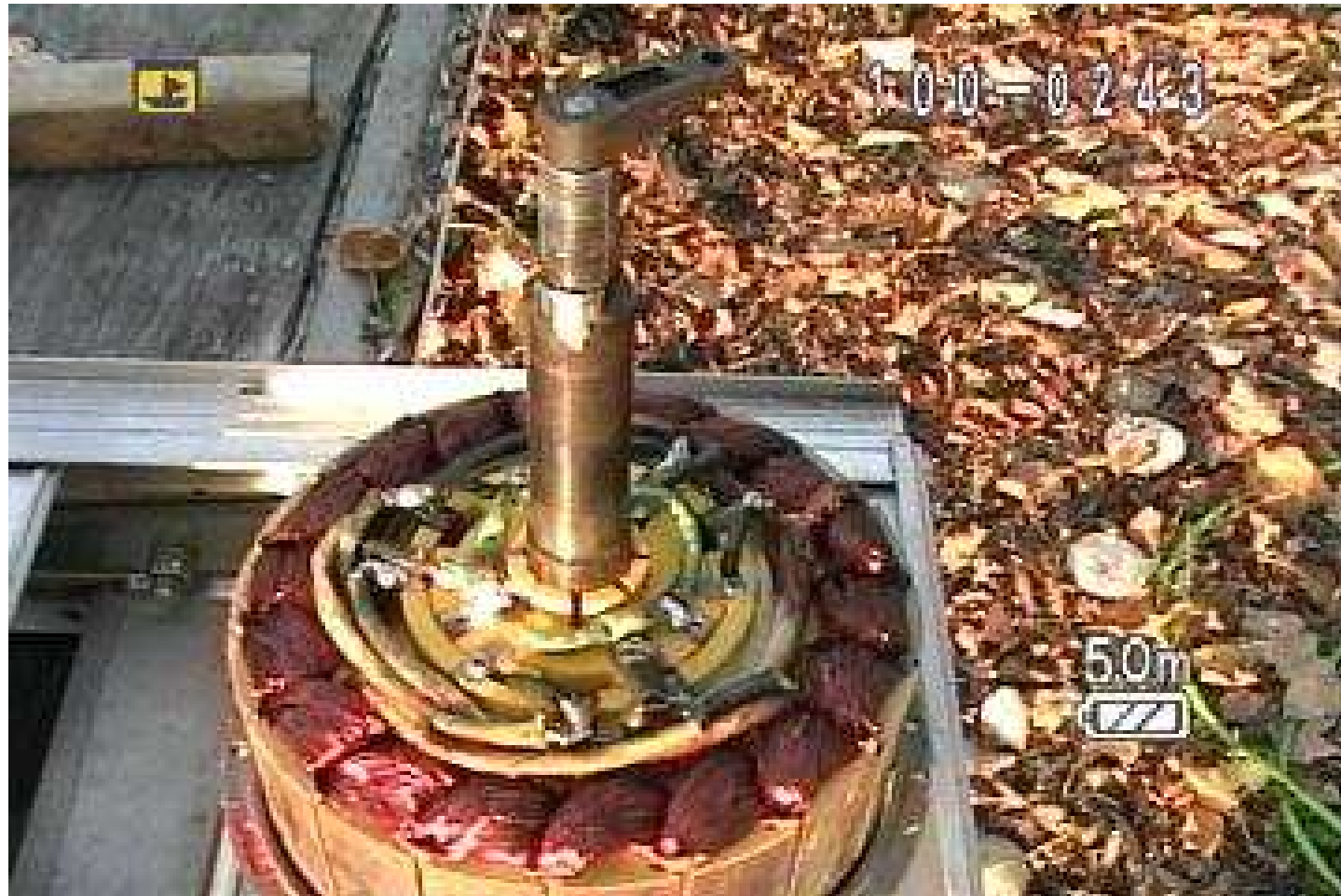
17 – Armature winding and shift plate.
