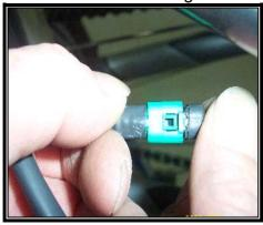
Caution!!! If insertion seems difficult, try again by slightly modifying the angle until the two connectors are perfectly aligned.
