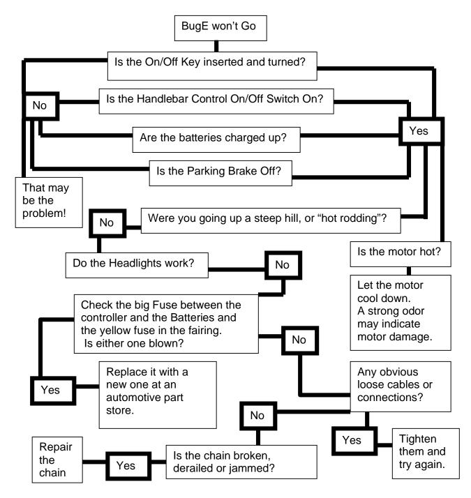
**CAUTION:** If the BugE still won't go, You may have a bad Controller, Throttle or Motor. Contact the manufacturer. **BASIC 48 VOLT WIRING DIAGRAM**
