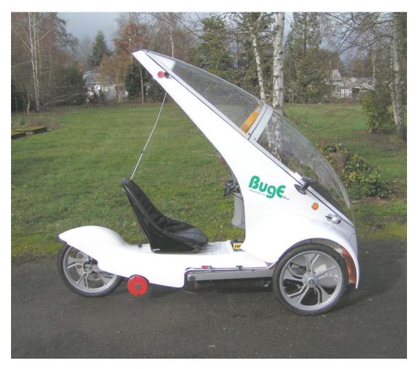
The **Seat** should be positioned for the comfortable use of the primary driver. The seat can be repositioned by removing and re-installing it in different mounting holes.
