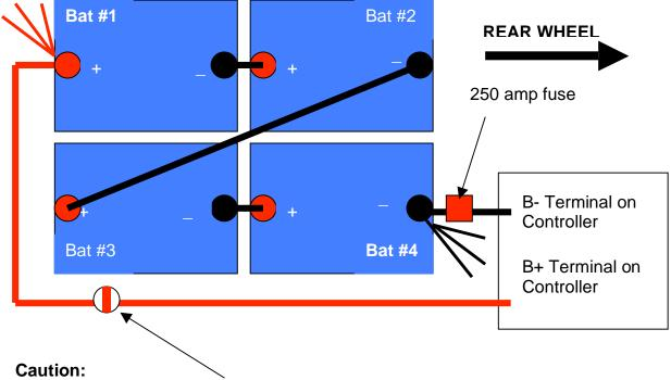
Always turn off the key switch before connecting batteries.
