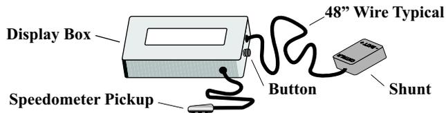
For operation, the shunt must be connected directly in series with the positive and negative leads of your vehicle's battery pack. It is recommended that the shunt is placed after any series switch or fuse so that the meter powers down when the pack is shut off. The correct polarity and orientation are embossed in the molding. In the event that the polarity is accidentally reversed, the meter will not power up. An internal diode protects against damage from reverse voltages.
