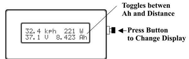
A quick press of the button will toggle to show other display screens of interest. The 2nd display shows just the electrical statistics from the battery pack, including the current in amps. This is the default screen for the non-speedometer model.
