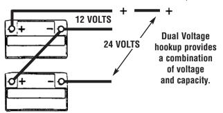
To properly recharge, a sophisticated "battery isolator" should be installed. Otherwise, one battery will be continually overcharged and the other undercharged in a dual-voltage set-up.
