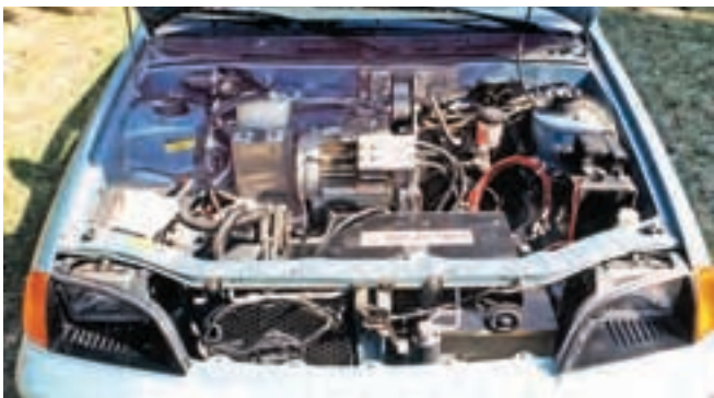
Solectria Force EVs were built on the engineless bodies of brand-new Geo Metros.
