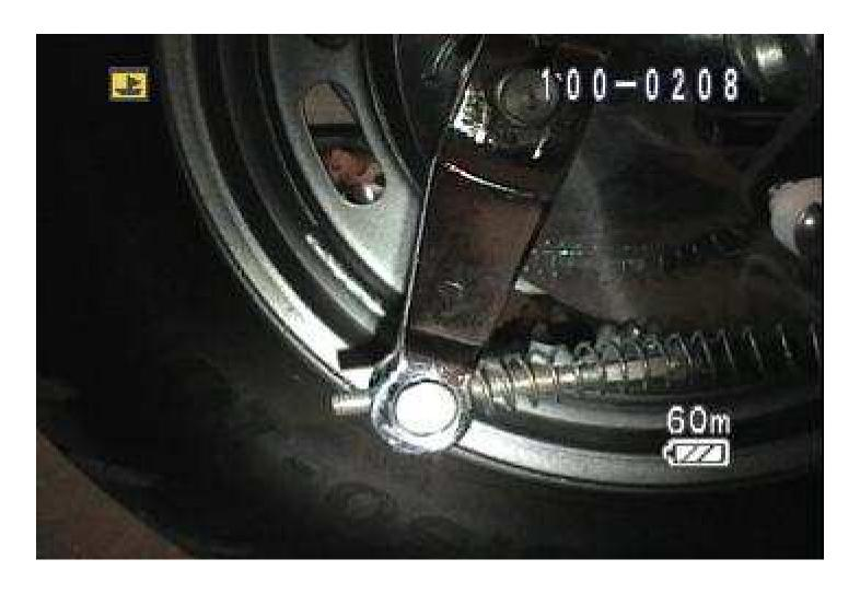
11 – Do NOT remove the brake barrel bearing or linkage yet, but take care the barrel does not fall out and roll away.
