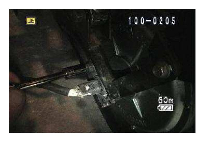
8 – Remove the 10mm bolt from the axle safety strap.
