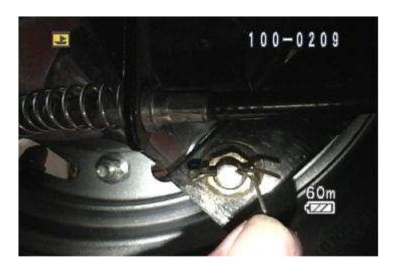
12 – Locate the drum brake retainer bolt, remove the cotter pin, nut and bolt.
