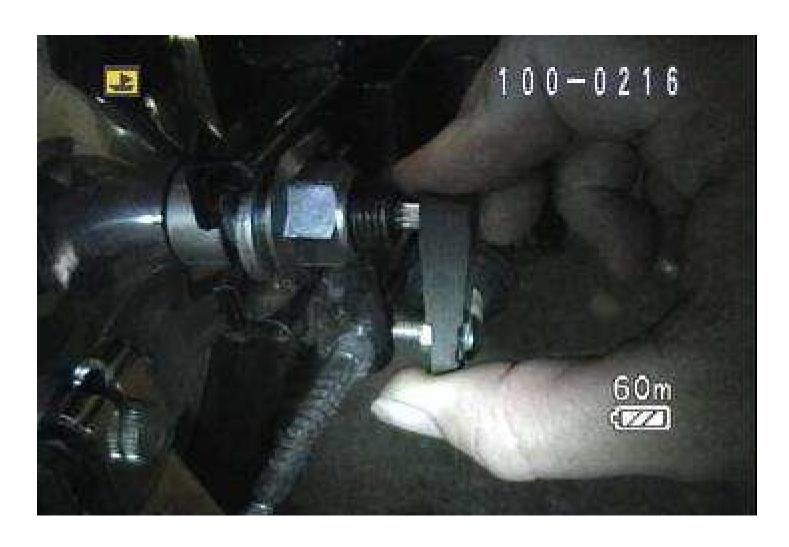
19 – Carefully work the black shift lever off the splined shift shaft.
