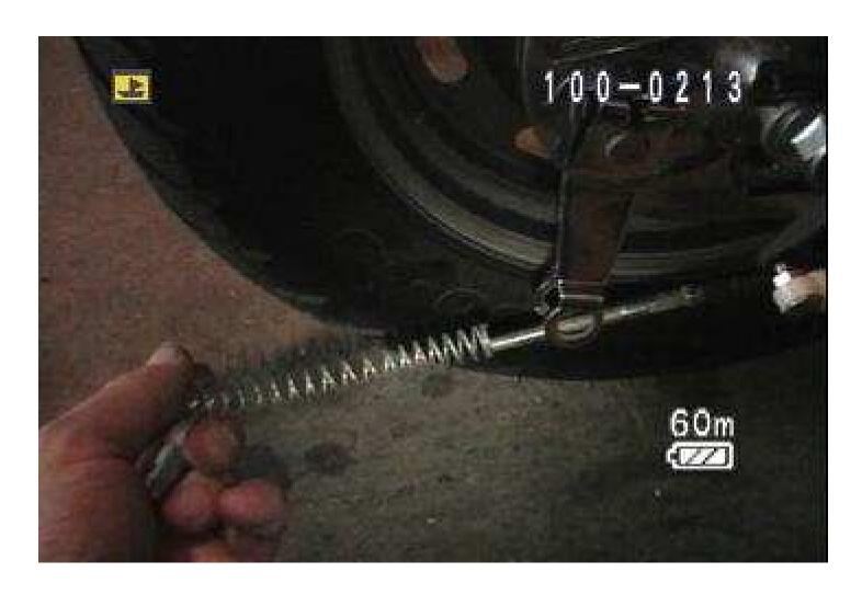
16 – Remove the brake linkage return spring.
