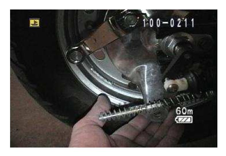
14 – Rotate the drum backwards and remove the brake linkage from the barrel bearing.
