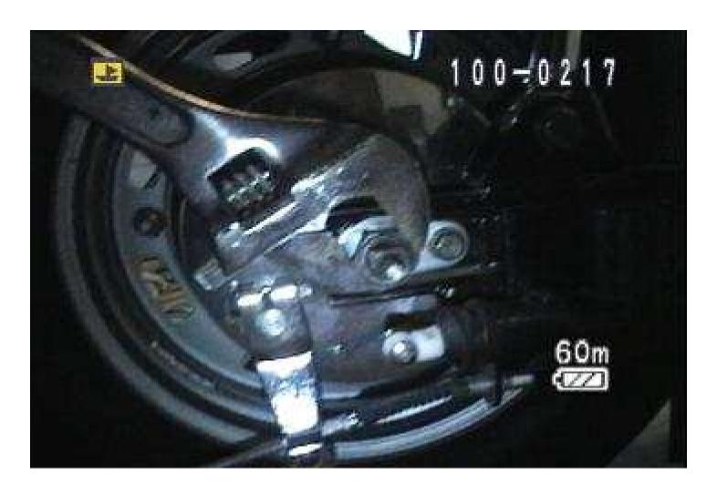
20 – Loosen the right axle nut, if tearing the motor down, remove the axle nut. Remove the 10 mm bolt from the axle safety strap.
