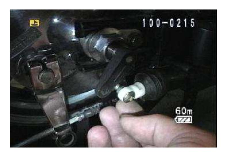
18 – Once the shift linkage is removed manually slide the linkage back towards low speed.
