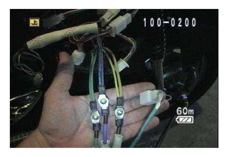
3 – Remove the screws and nuts that hold the motor wires to the controller and unplug the 5 wire HALL sensor.
