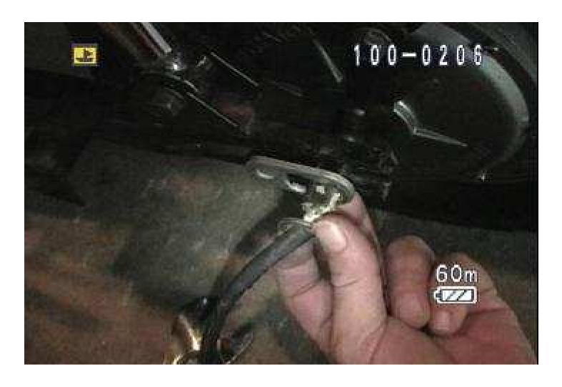
9 – Slide the axle washer and axle safety strap away from the swingarm.
