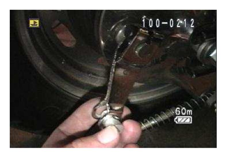
15 – Remove the brake barrel bearing.
