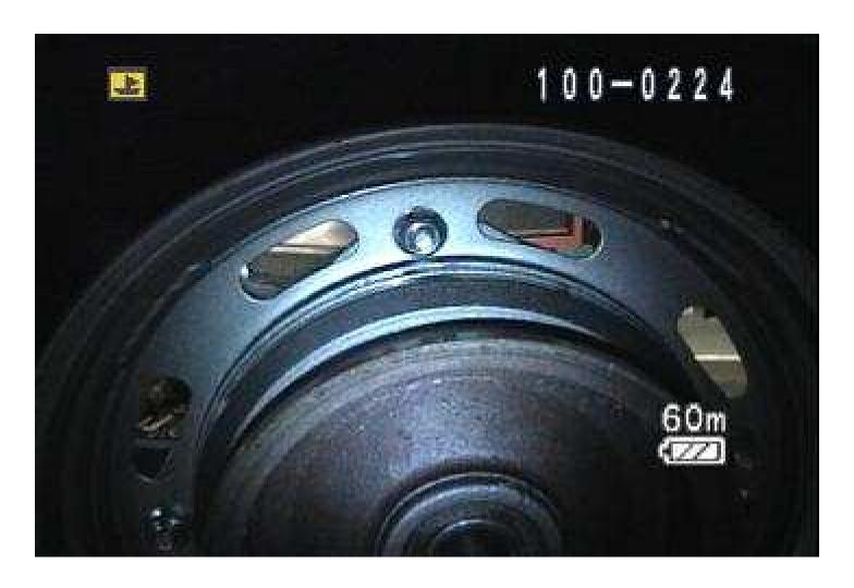
27 – To remove motor from wheel, use a 10mm and 12mm ratchet, two ratchets needed, remove the four nuts and bolts that hold the motor to the wheel.
