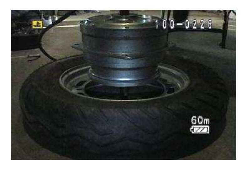
29 – Done, when reassembling, make SURE the tire valve stem is on the shifter side of the assembly and NOT the motor wire side of the assembly. If changing tires, pay attention to wheel direction arrows stamped on the side of the rubber tires
