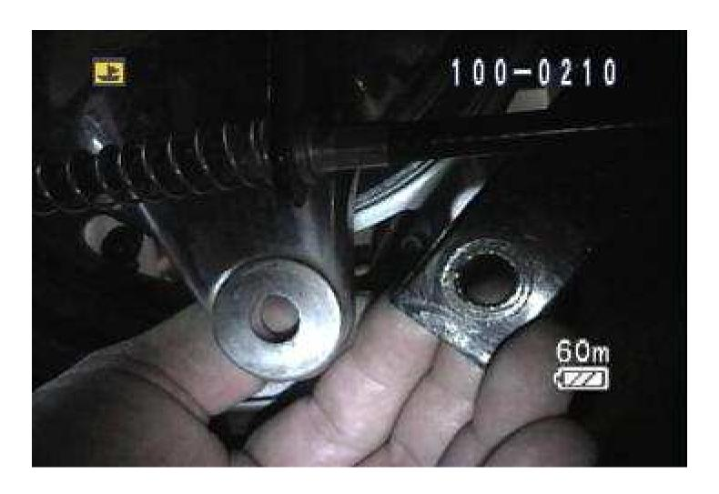
13 – With the drum brake retainer bolt removed the drum will now spin freely back and forth.
