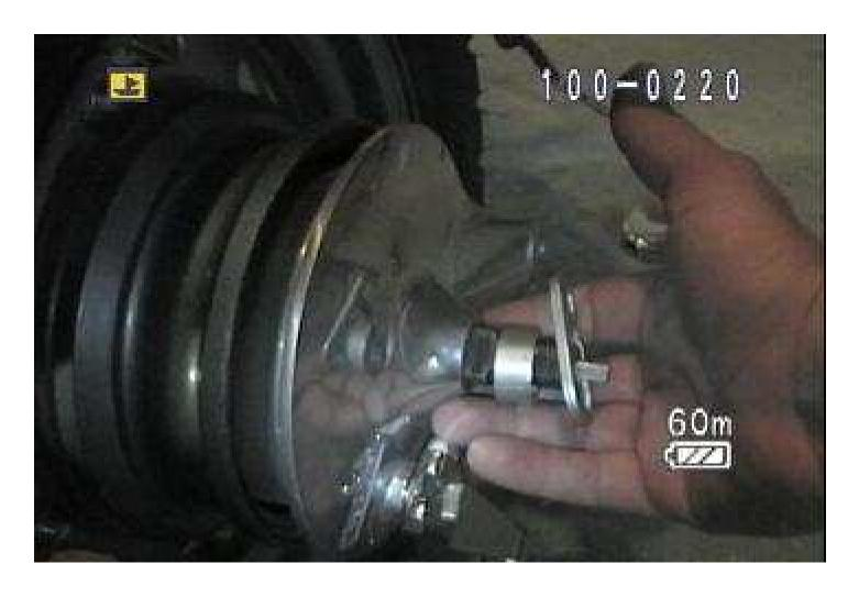
23 – Remove the safety strap, bushing and brake drum from the axle.
