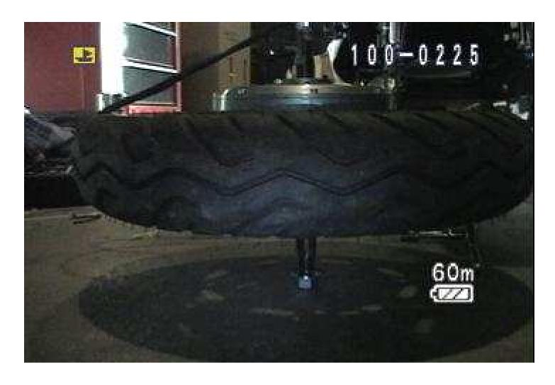
28 – If the motor is tight in the wheel, set on end ONLY IF THE AXLE NUT IS PROTECTING THE SHIFT SHAFT END and give the tire an even whack.
