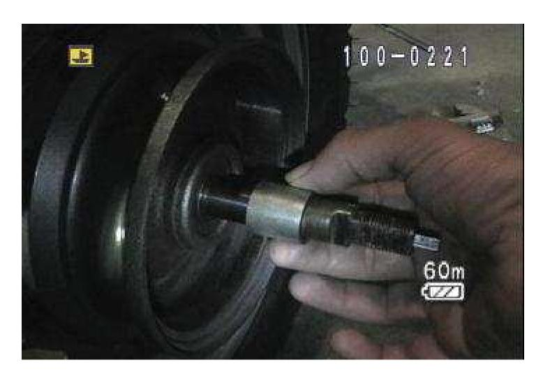
24 – Remove the wheel to brake bushing.
