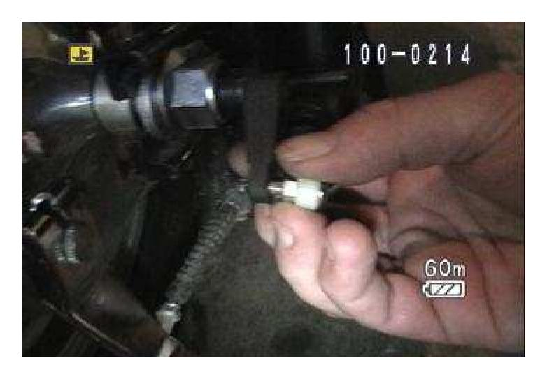
17 – Fully extend the shift linkage into high speed and carefully work the coupling screw out of the black shift lever. This screw normally is not threaded into the black shift lever but just pressed in place.
