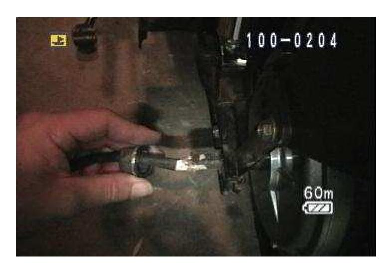
7 –If you intend to tear the motor down then remove the axle nut completely.
