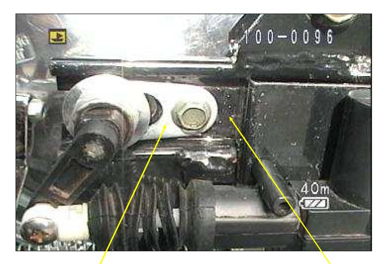
8- The rear axle safety retainer, notice that the rear of the selenoid housing mounting bracket is UNDER the right axle safety retainer, this is going to be changed. We are going to slightly loosen but not remove the right axle nut and remove the nut and bolt that hold the selenoid housing on the bike.
