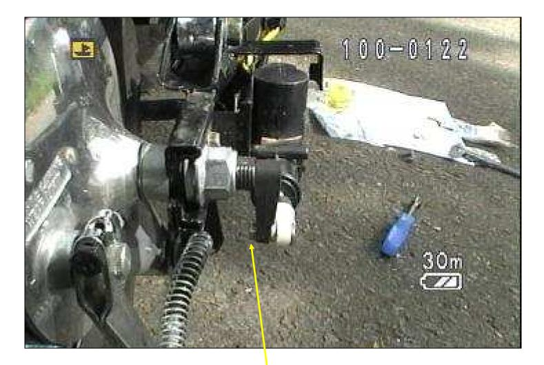
32- You will want to add a small locknut or a thin nut with some locktite on it to hold the selenoid head screw in. Don't tighten the nut or the shifter will bind, just enough to secure the screw is all that is needed.
