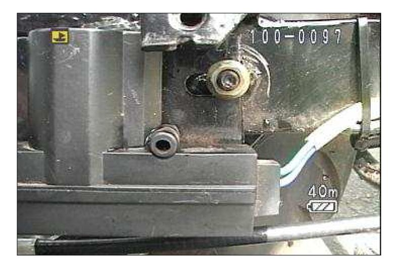
9- The nut on the right side of the selenoid housing, remove this.
