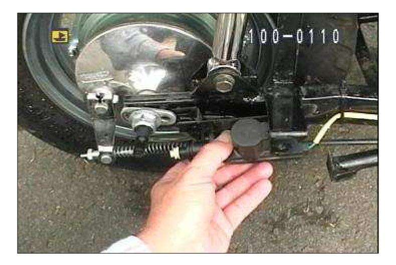
17- With the selenoid housing nut and bolt removed and the selenoid plunger removed from the plunger head, slide the axle safety out of the way and remove the selenoid housing out of the way.
