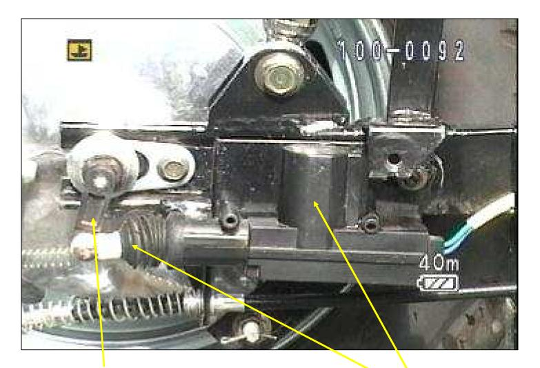
3- Gear shift arm is moved back and forth by the selenoid plunger. Plunger moves in and out of selenoid housing by servo motor. The gear shift arm pictured is not correct, the selenoid plunger is retracted for low gear, the arm should be just to the right of straight down, or striaght down, it is instead left of straight down.
