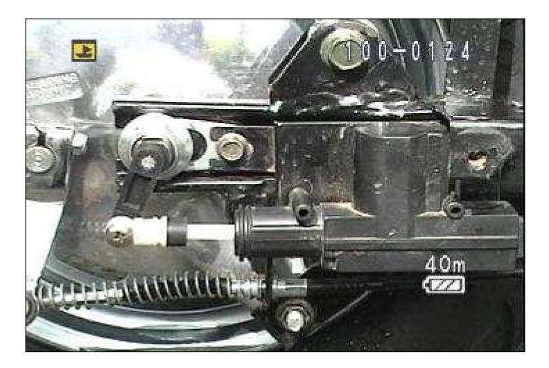
19- It will help if you know where we are going with all of this, when we remount the selenoid housing, we are going to place it ON TOP of the axle safety instead of under it. This will do two things for us. It will move the selenoid plunger outward inline with the gear lever, and allow for easy back and forth adjustment of the gear shifting mechanism.
