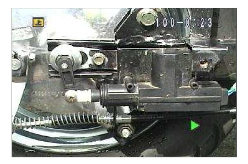
30- Reassemble, note the shift plunger is retracted (low), the shift lever is just to the right of straight down, or straight down. It should NOT be anymore to the right of straight down than pictured. Also the selenoid housing is now adjustable from right to left by loosening the housing bolts, make sure you start with the housing centered, THEN adjust the lever so it is right of down or down. Then adjust the housing for good shifter movement.
