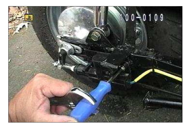
10- This special tool is known as a West Virginia Socket Set. Use it to remove the nut and bolt from the selenoid housing.
