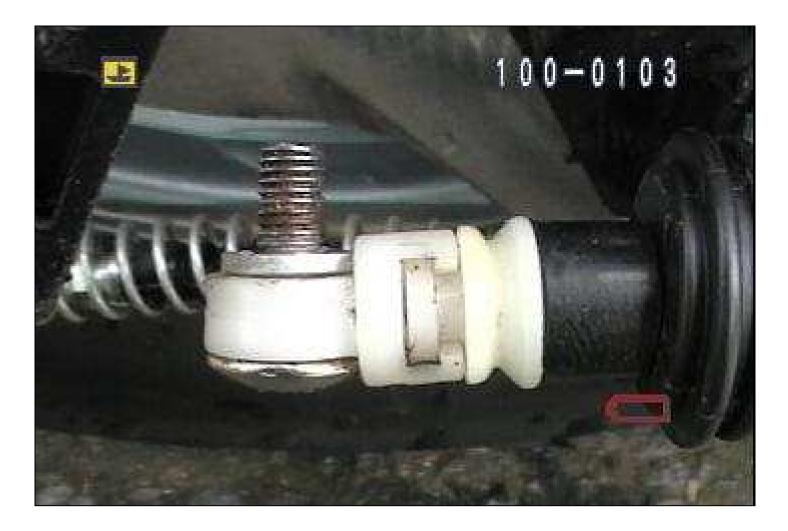
16- Closeup of the head and plunger, note the washer your bike will NOT have, as well as the possibly longer screw that your bike may not have. More on this in a moment, but the washer is added as a bearing surface and to prevent binding which WILL OCCUR if you do not add this washer. The washer requires some special fabrication.
