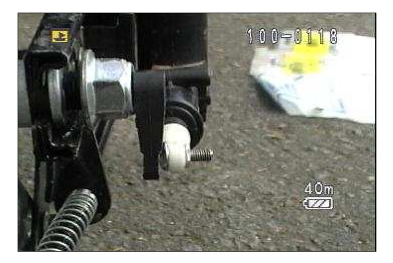
26- Test fit and examine the linkage, this one is not even touching the lever, so I went for a thinner washer on the rear housing (bolt) so it would sit a tad closer to the lever and be more inline.
