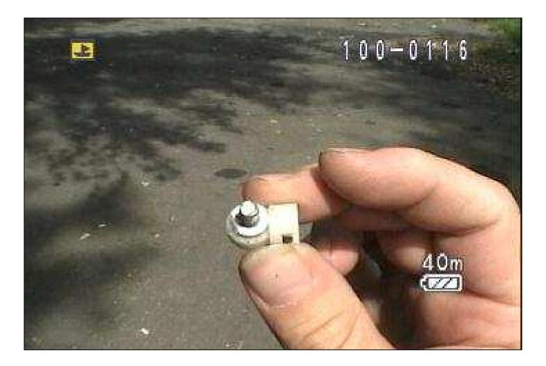
29- Go find a 1/16 washer (thick) and grind a small flat edge on one side, once you test fit it things will become apparent. If you do not have a grinder, hold the washer in a wrench and slide the edge on a concrete sidewalk and it will grind down just right, that's how we made shivs in elementary school during recess, remember ?.
