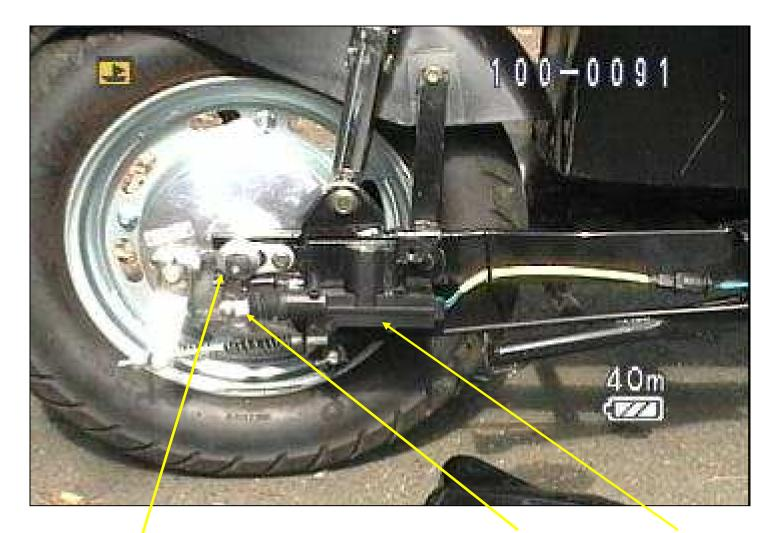
2- With the cover removed we can get to the shifter linkage, selenoid and right axle bolt
