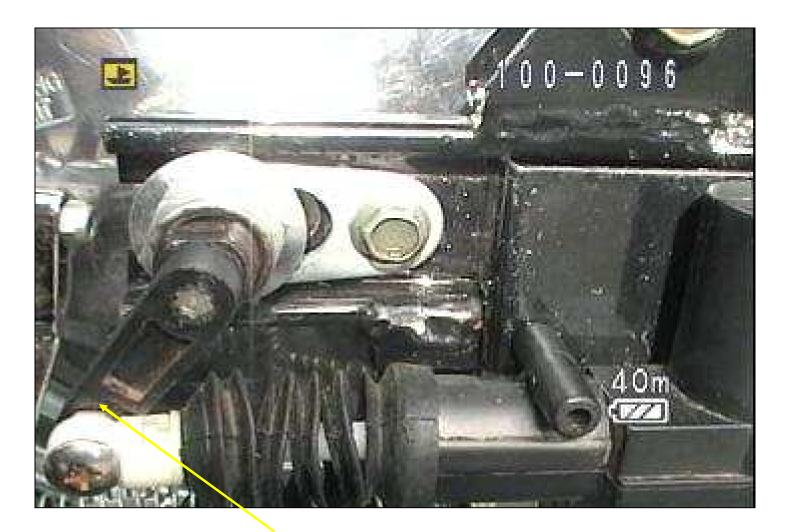
7- The plunger fully extended. Your bike may have the plunger attached to the shift linkage on the inside, or as pictured here, on the outside of the shift lever. When we are done, it will be on the outside as pictured.
