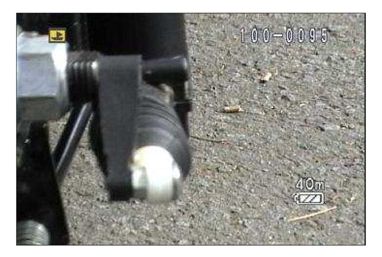
6- Another angle to show the misalignment between the selenoid plunger and horn. The added stress and friction the plunger must deal with in this configuration will shorten its life and cuase shift problems.
