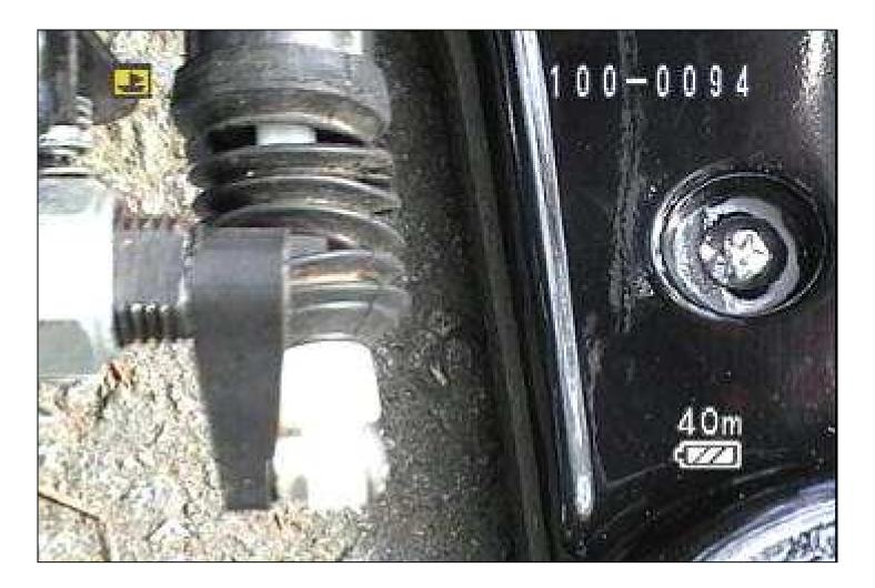
5- The plunger has been fully extended to place the bike in high speed mode. Notice the protective boot has deteriorated in only 6 weeks of exposure to the elements. The boot is very poorly made and not UV resistant. It will be discarded until a replacement solution is sourced.
