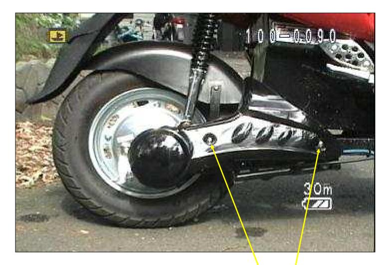
1 – Remove the plastic right cover, held on by two phillips head screws.
