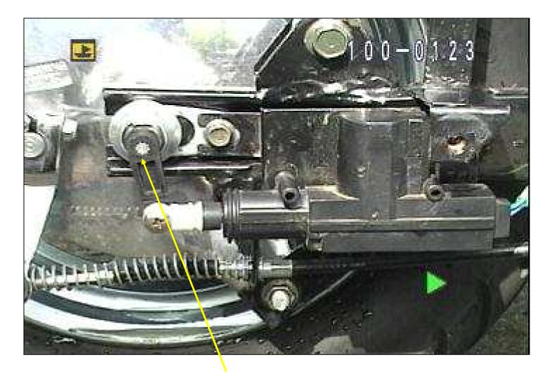
31- If you can't get the shift lever right of down or down without radically sliding the house, pull the shift lever off the spline and flip it over and try again, it is slightly offset when flipped over.
