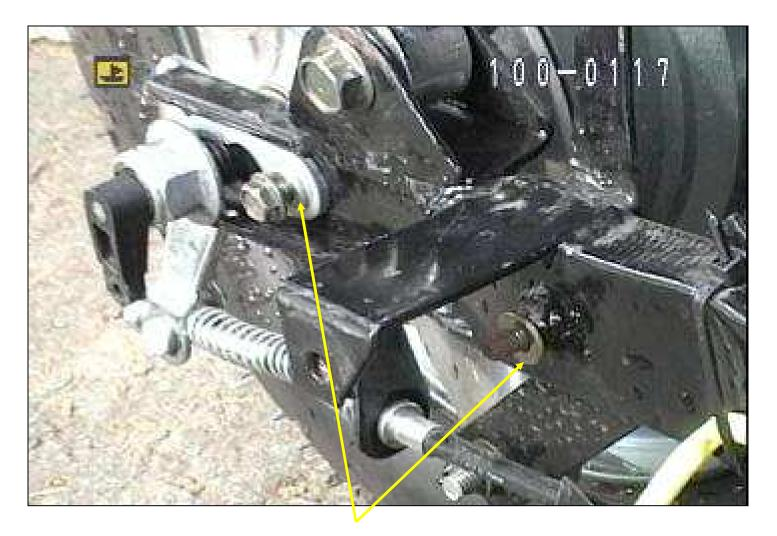
25- Add two washers to the bolt and nut for the housing, I used thin on the rear (bolt) and thick on the front (nut). When the housing in reinstalled, it will sit ON TOP OFF these washers.
