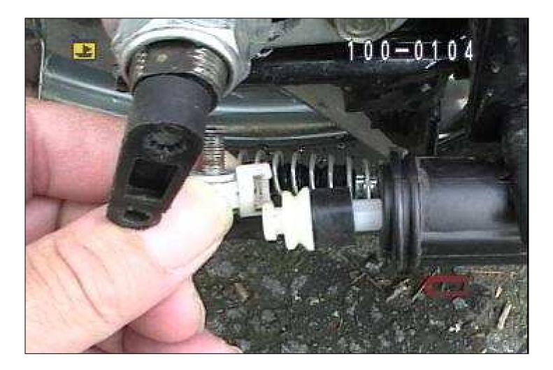
15- Once the head is disconnected from the plunger, removing the head from the black shift lever is painless, should just slide out as the screw in the head that goes into the black lever is just slid in and not threaded in as one might think.
