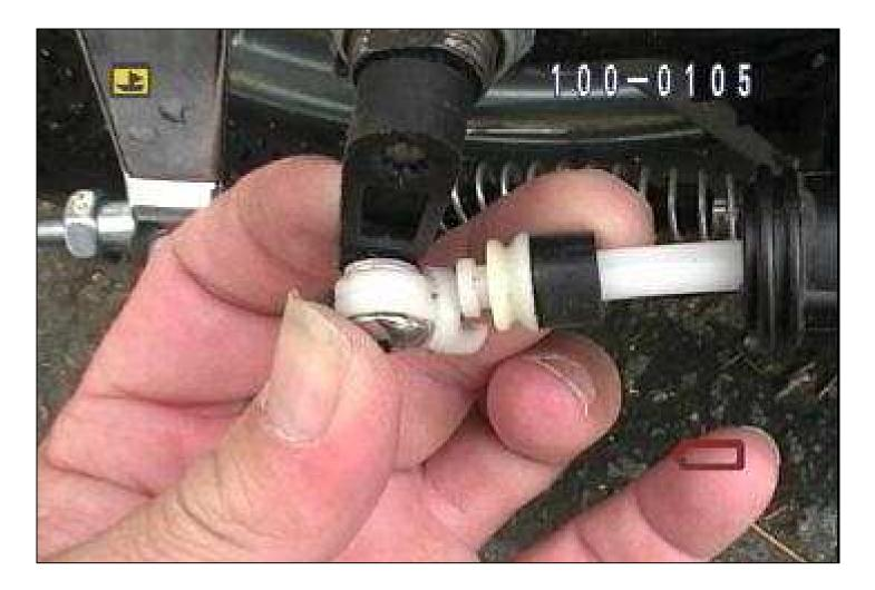
14- The shift plunger head and the shift plunger just snap together and apart.
