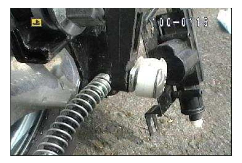
28- Now, see the silver washer between the white selenoid head and the black shift lever ? Pretend it's not there, because on your bike, it's not. Look at the lever just to the top of the washer, see that ridge that jumps out in the black plastic, if you do not add a shim here, the shifting will not work right. But you can't just add the washer, it will not fit, it needs a little work.
