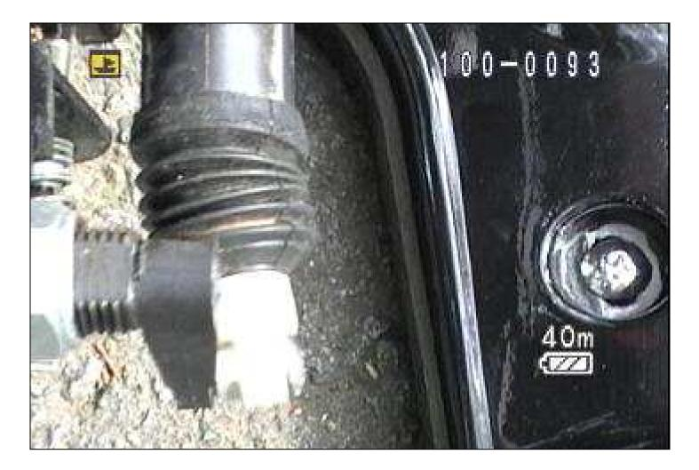
4- As delivered from the factory, the selenoid plunger is stressed and bent due to poor alignment with the shifter arm. To correct this, we will shim the entire selenoid housing further to the right to remove the stress, the added benefit to this will be you can add an adjustment capability to the selenoid mechanism that does not exist now.
