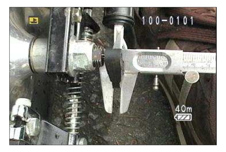
23- The shift lever is 3/16 of an inch thick, that is approximately how far the selenoid housing must be moved outward to achieve one of our goals.
