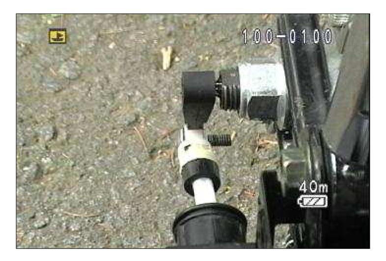
22- Lets review one of our goals, when the selenoid head is removed from the shifter lever and allowed to go where it wants, it is perfectly in line with the lever, which is WRONG, it need to be on one side or the other, for our fix, it MUST be on the outside. But how much to move it ?
