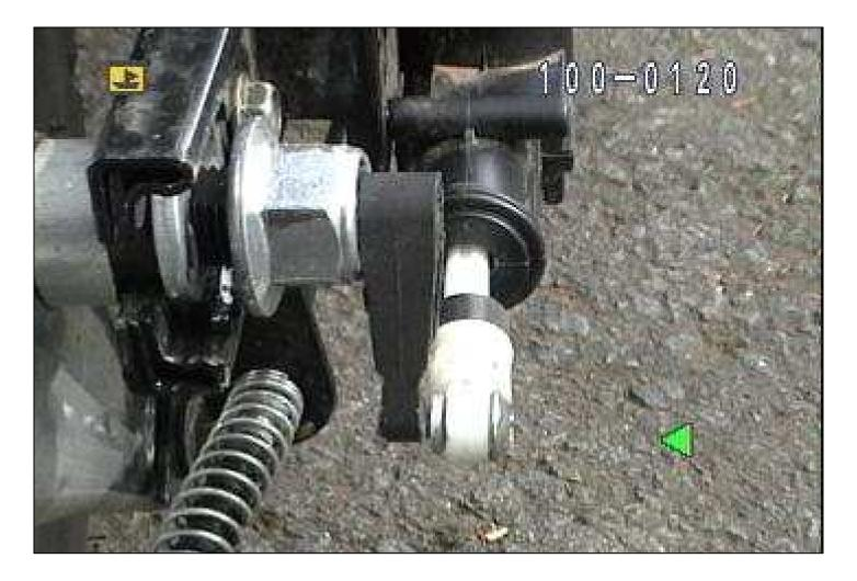
12- This bears repeating, do NOT run the axle nut into the shift arm lever or you may break it. We only need the axle nut a couple of turns loose.
