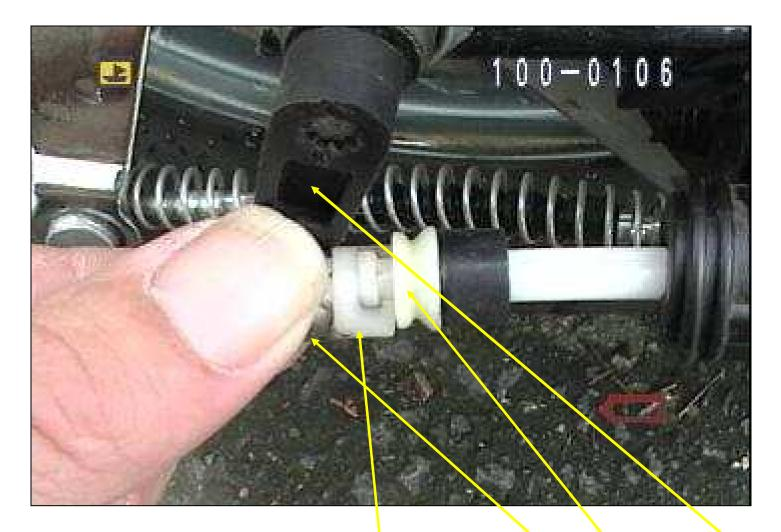
13- Instead of forcibly removing the linkagepivot screw out of the shift lever, disconnect the shift plunger head from the shift plunger.
