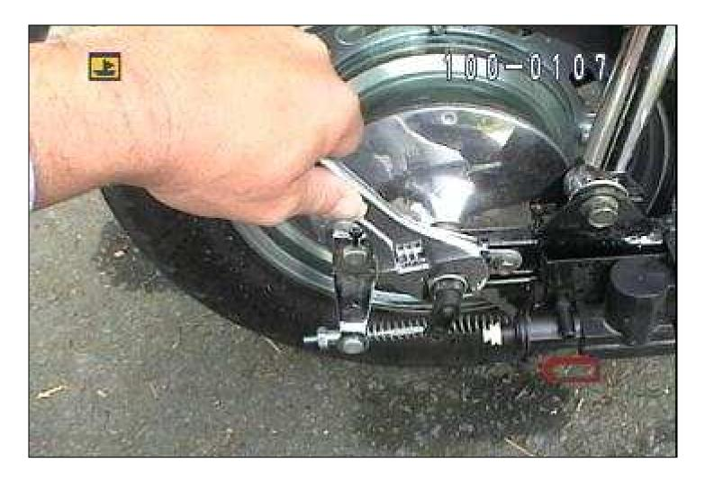
11- Loosen, but DO NOT REMOVE, the right axle nut, take care no to run it up onto the gear shift lever.
