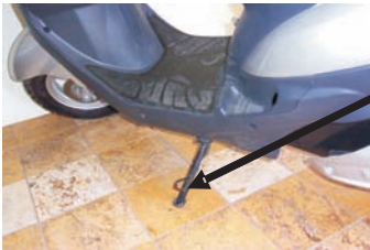
Kick Stand (this automatically cuts off the power so the bike will remain stationary)
